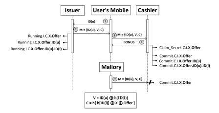
Fig. 5. Capturing Hash-based NFC M-coupon requirements
