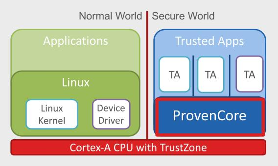
ProvenCore pushes to the extreme. Secure Apps are not trusted by the kernel and they are isolated. The kernel is small enough to prove integrity and confidentiality properties.
